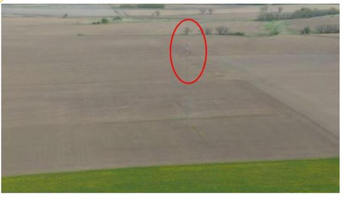
MET towers or Meteorological towers are used to gather wind data necessary for site evaluation and development of wind turbine projects. They can be erected very rapidly and may be on site from a few days to up to a year or longer. At this time there is no standardized notification system in place to indicate when and where these towers are erected.
